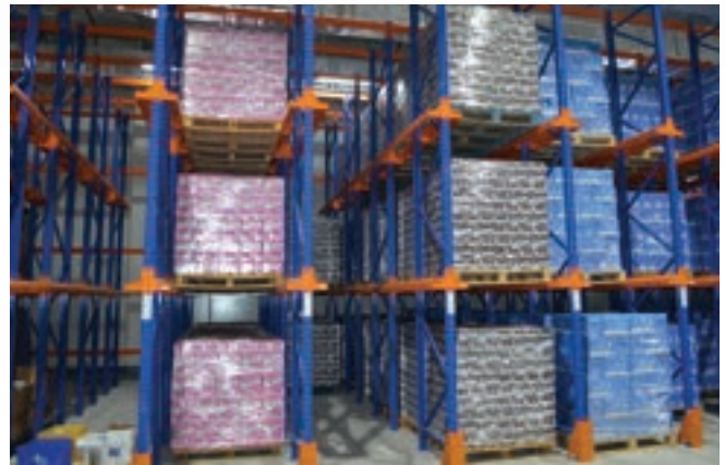
Drive In / Drive Through Racking
